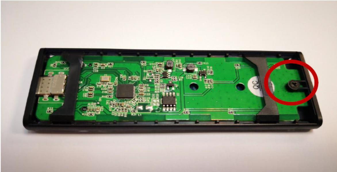
**Step 6: Remove all double-sided tape liner which is placed on the cases, positions as shown for correct upper & lower case.**
