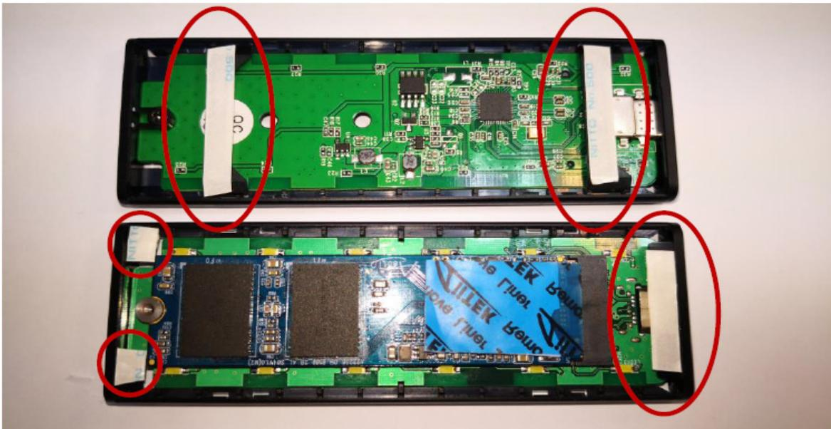
**Step 7: Place the upper and lower case and the positions of the cassette are as shown**
